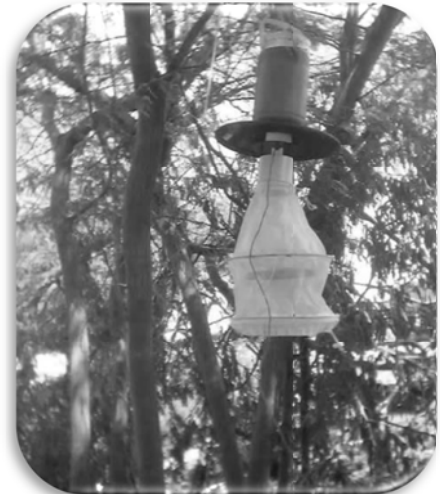
Mosquito traps, used for vector control and monitoring Picture © Ministry of Agriculture, Kingdom of Saudi Arabia
